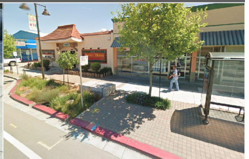
Bioretention curb extension and suspended pavement system integrated with bus stop, Castro Valley (from Google Earth)
